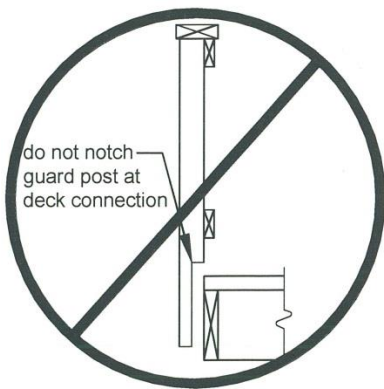
Post Notching Prohibited
